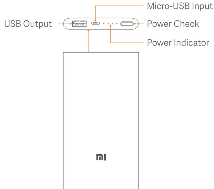
The Power Check button is not a Power button.
